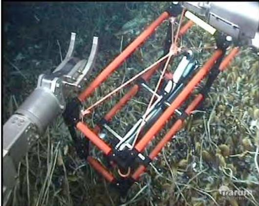
Fig 3. The Eddy correlation system by Frank Wenzhöfer (MPI) to measure integrated oxygen fluxes is placed on the mussel bed.
