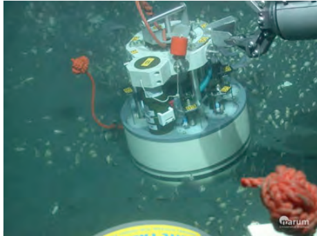
Photo 1: Respiration measurements on field of vesicomyid clams with the benthic chamber CALMAR of IFREMER
