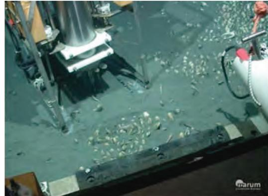
Microsensor profiler deployed close to a clam patch
